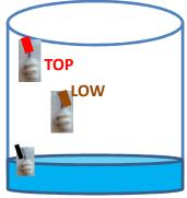
STATUS: when the water in the tank once reaches the top level, the motor will stop. The top and bottom level will start glowing OHT TOP: yellow led GLOW OHT LOW: red led GLOW
